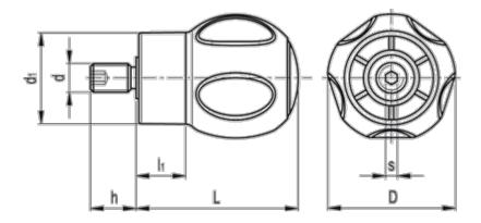
$\begin{array}{lll} D & = 50 \\ d1 & = 36 \\ d \ 6g & = M10 \\ h & = 17 \\ L & = 62 \\ l1 & = 19 \\ s & = 5 \\ Weight \ (g) = 90 \end{array}$
